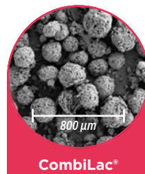
Figure 5: SEM image of MEGGLE's CombiLac® by ZEISS Ultra 55 FESEM (U=5 kV; Au/Pd sputtered).
